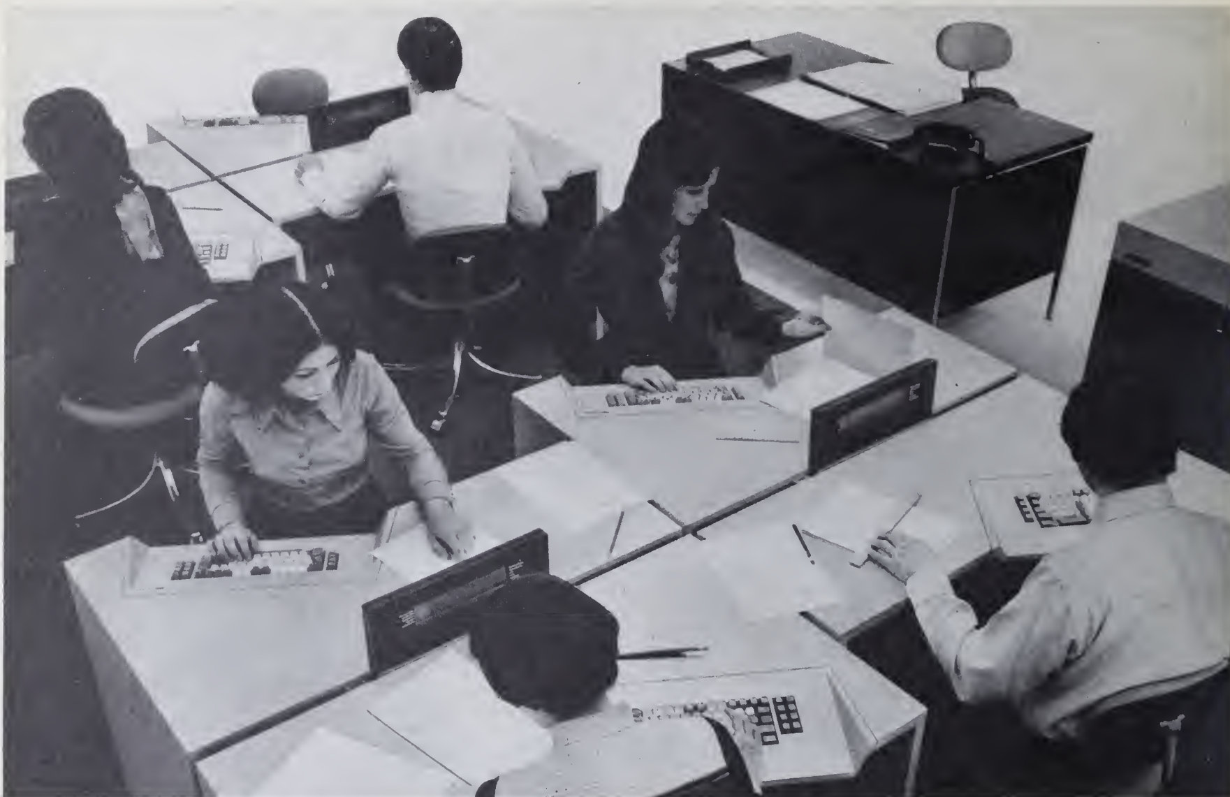
A sloped keyboard, a sharp, bright display panel and quiet operation are some of the human engineering factors enhancing 3760 productivity.
